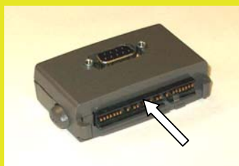
Alignment Notch Moved Inward
