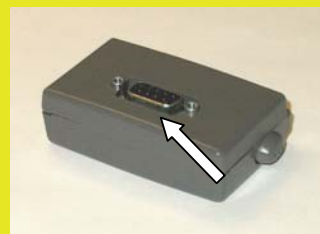
Power Connector Removed
